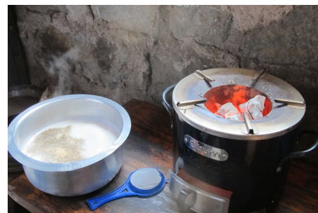
The ash tray can be used to control the heat from a jikokoa
