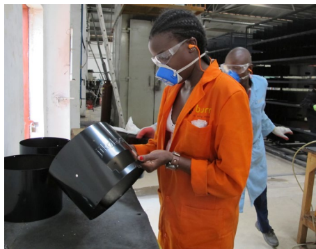
Quality inspector Cindy checks the cladding for a jikokoa before final assembly.
