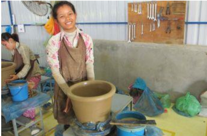
Producing clay pots for ceramic water filters (Hydrologic factory, Cambodia)
